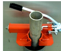
3" Steel Pipe on 8" Casing
