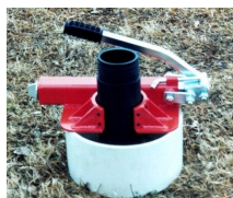
4" HDPE Pipe on 12" Casing
